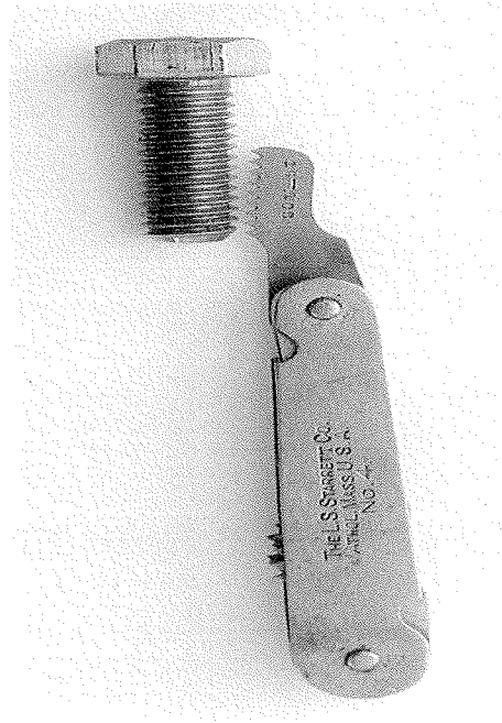
Fig 1.5: Measurement of pitch or threads/inch
